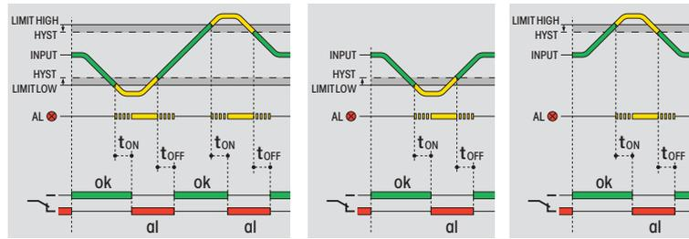
gn ok ye fail rd alarm Alarm delay: tOFF, tON
